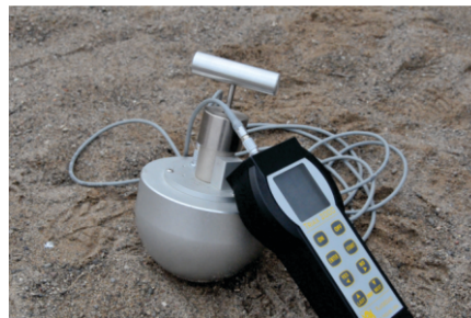
Manual Drop Device attached to the TRIAX 2015 Head Form (Not Included)
