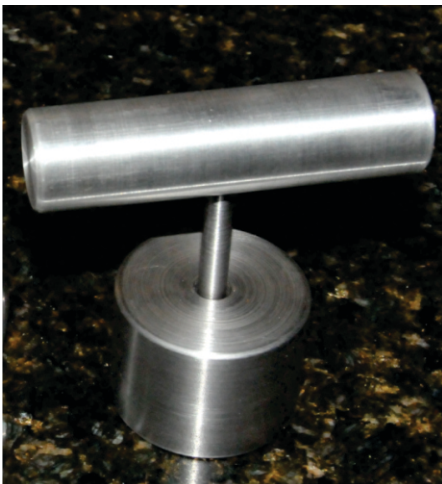
Manual Drop Device attached to the TRIAX 2015 Head Form (Not Included)
