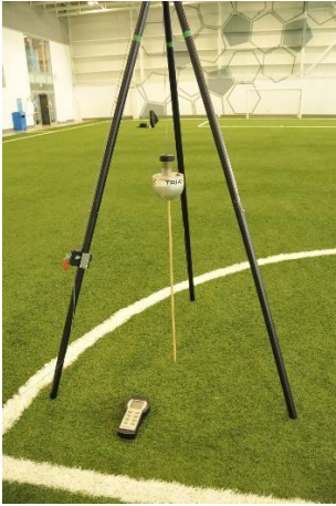
Three drops from the same height to the same point with measuring rod
