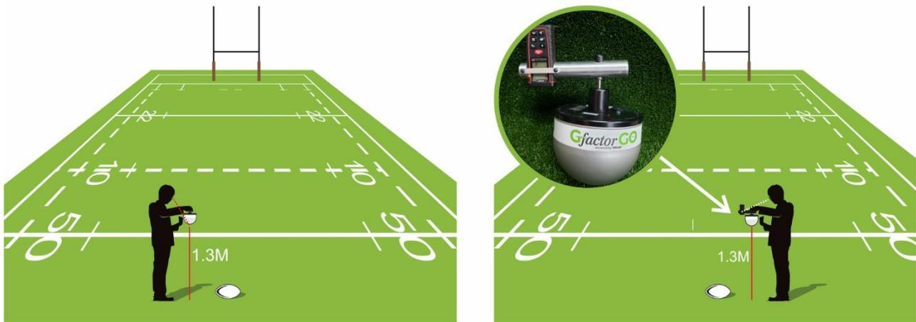
The operator ensures the drop height is greater than 1.3M, either by "eyeballing" or using the laser distance finder.
