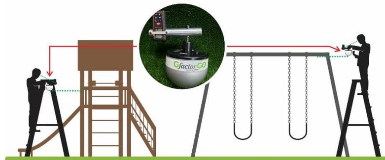
1. Find the fall height or height above the drop height the test is to be performed from. In this example, for the structure, the owner has selected the drop height at the top of the barrier, while the drop height for the swings remains at the fall height of the pivot point as in ASTM F1487.
