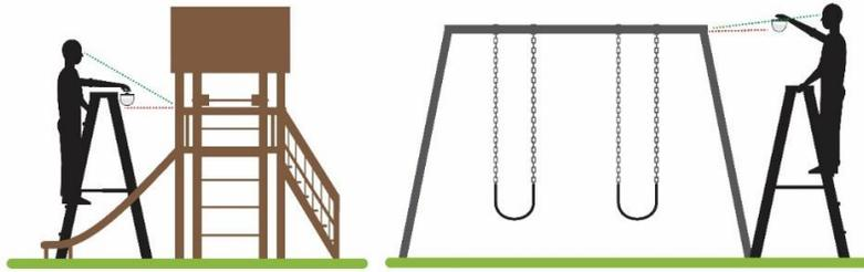
The operator of the *GfactorGo* determining drop height with the laser distance finder
