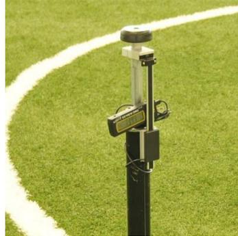
Once the reading is taken the operator once again places a hand or foot on to the base plate of the depth gauge and then retracts the 3 prongs by pulling on and raising the centre rod until the exposed rods are fully retracted.
